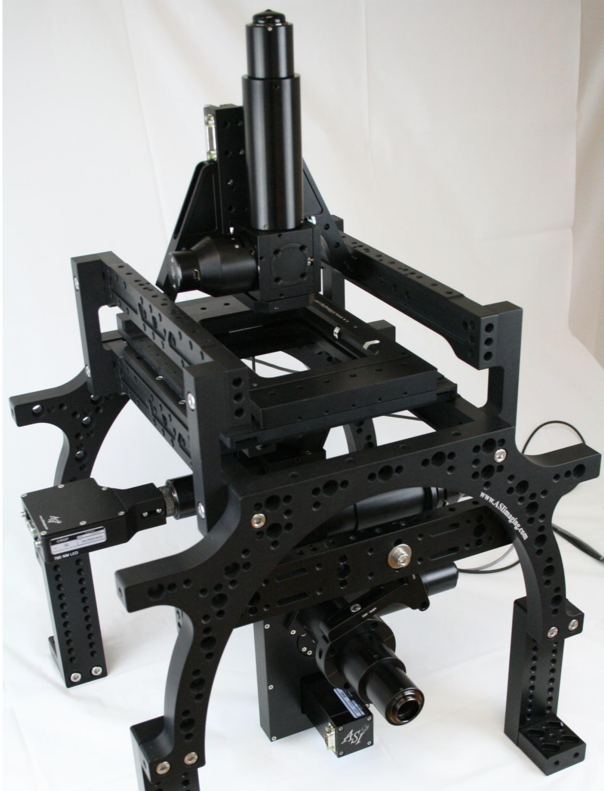
Figure 11: Double microscope with piezo-Z stage CRISP and filter wheel on a RAMM-DV frame with STILTS .
