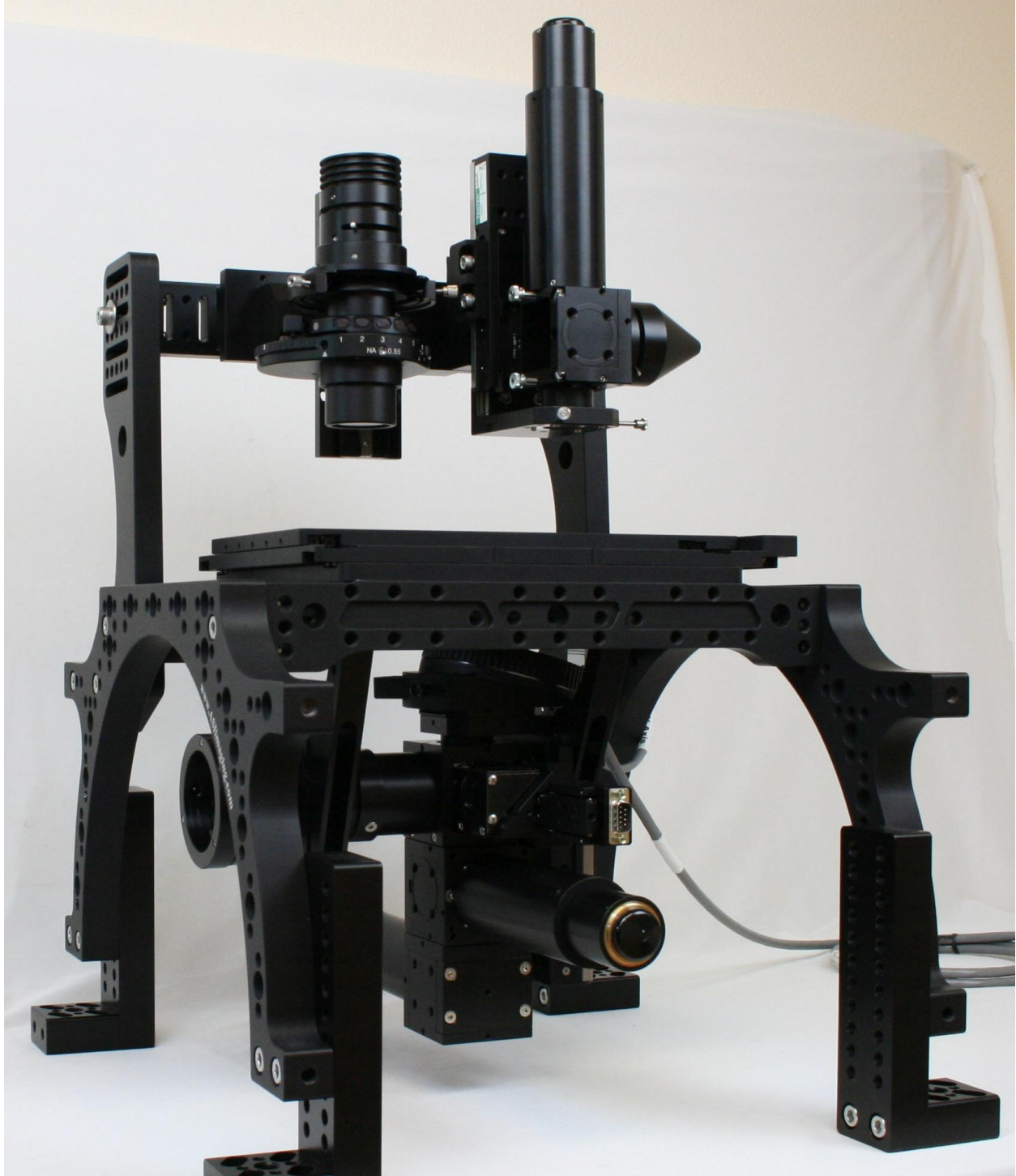
Figure 4: RAMM-DV frame microscope with three vertical cubes and a manual nosepiece. Below the nosepiece is a four-position automated filter slider, below which are cubes for two camera ports. This system has a transmitted light condenser and another microscope mounted to a top-side slider. Either the condenser or the microscope can be place directly over the bottom-side objective.
