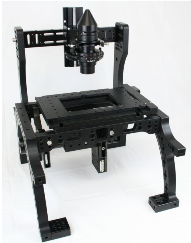
Figure 1: Basic RAMM inverted microscope with automated stage and trans-illumination.
